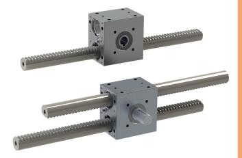
The rack jacks are available with one or two racks. In the double version, the racks move in opposite directions.
